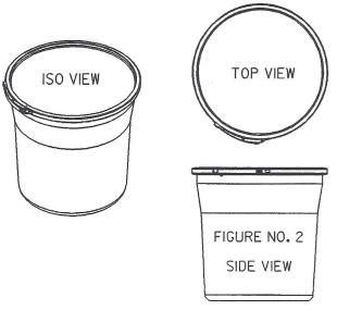
PLace the lid on the drum and center the lid on the drum by tucking the drum flange inside of the lid gasket area.
